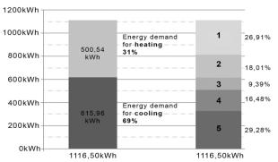
Figure 12: Reasons determining a building's energy demand in the case of Milan. 1-Heating loss through window, 2-Heating loss through wall, 3-Cooling demand due to heat transport through the wall, 4-Cooling demand due to solar irradiation through the window, 5-Cooling demand due to internal thermal load.
